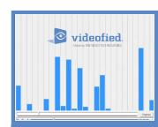
The video frame shown above is of a Videofied message being transmitted across many different frequencies (spread spectrum). If there is interference or "jamming" on a frequency, the system works around it to find an open lane to transmit the message/video of the alarm.
